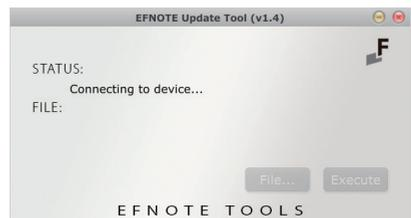
When the connection is established, the status shows “Device connected,” and the sound module shows following screen.
