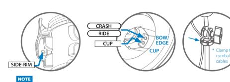
$\mbox{\ensuremath{*}}$  To avoid disconnecting the trigger cables unexpectedly, tie or clamp the cables.
